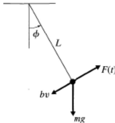
Figure 12.1 The three important forces on the driven damped pendulum are the resistive force with magnitude  $bv$ , the weight  $mg$ , and the driving force  $F(t)$ . (There is also a reaction force from the pivot at the top, but this contributes nothing to the torque.)
