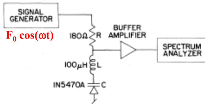
FIG. 1. Experimental apparatus for subharmonic generation.
