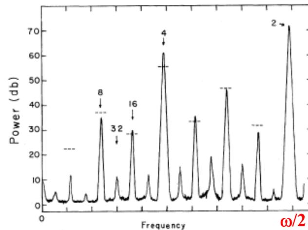
FIG. 5. Power spectral density (dB) vs frequency for  $f = 98$  kHz, dynamic range 70 dB, showing sub-harmonics to  $f/32$ . The components agree with prediction (dashed bars, Ref. 14) within 2 dB rms deviation, except for the peak at  $f/16$ .
