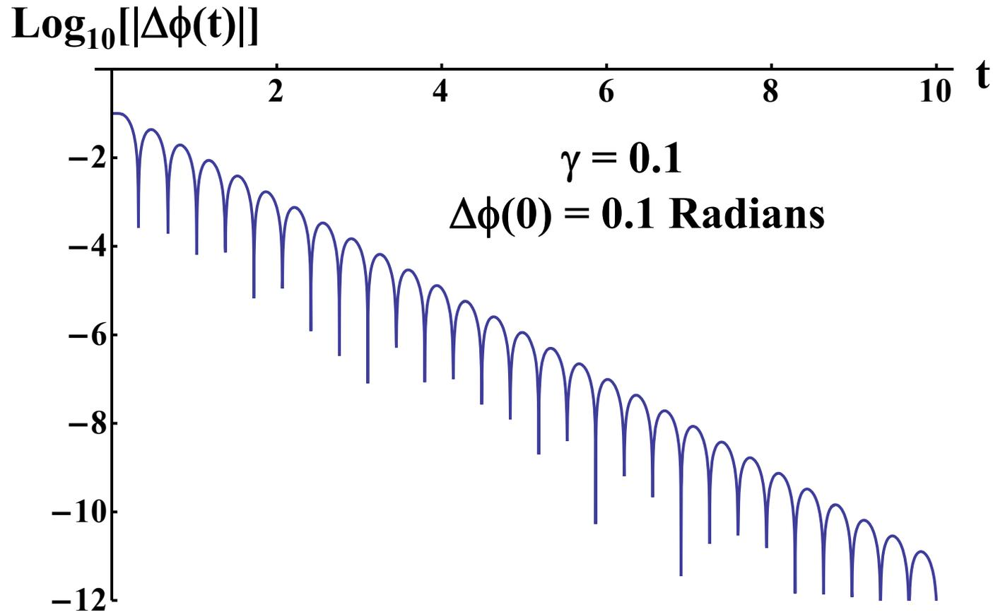
The trajectories converge quickly for the small driving force ( $\sim$  linear) case
