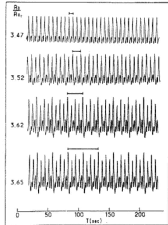
A period doubling cascade in convection of mercury in a small convection cell. The plots show the temperature at one fixed point in the cell as a function of time, for four successively larger temperature gradients as given by the parameter  $R/R_c$
